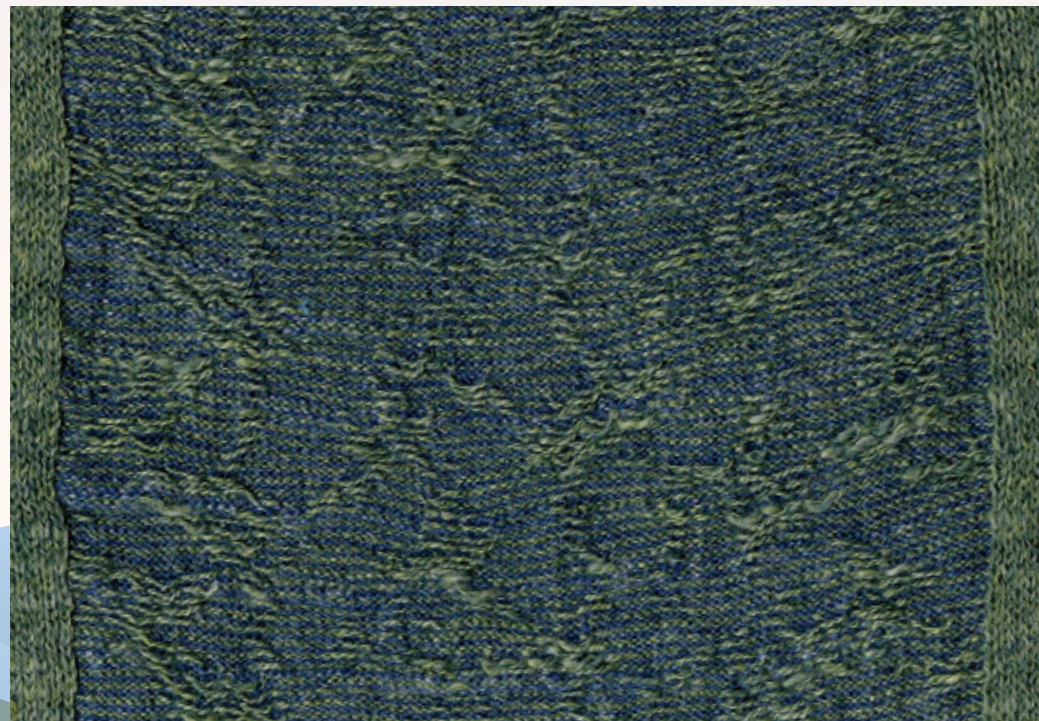
Product Name(产品名称): Rain Denim Heather Yarn, Uneven Budding Heather Yarn Content(成分): 100% Cotton(棉) Yarn Count(纱支): 20s/2 Yarn Lot(纱批): H222-104380-107, H120-Z100200-11 Color Code(色号): ES22283D, ES11808D Gauge(针种): 12gg, 1end Art NO.(花型编码): 210156
